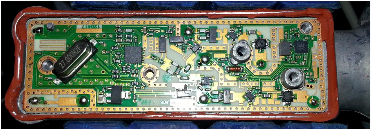
The PLL/Mixer chip is RDA3560m; a short data sheet can be obtained from <http://www.uhf-satcom.com/misc/datasheet/RDA3560m.pdf>
