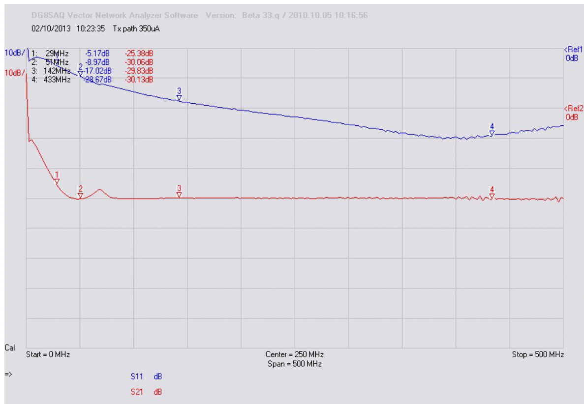
Figure 3 Network analyser plot of the Transverter Interface path on transmit (the red S21 plot). Note the broad constant attenuation above 100MHz. This can be varied by adjusting the diode forward current. S11 shows the Return Loss at the transmitter input. A value here of 17dB corresponds to a VSWR of about 1.3
