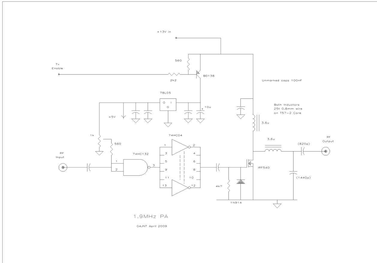
On testing a few big surprises came to light. The PA worked best at a frequency appreciably higher than it was designed for, giving maximum power at around 2MHz rather than 1.84MHz. In fact at 1.84MHz the output was rather messy, with some spurious / instability present. At 2MHz it was giving a very clean output and the power being supplied to the load was over 30 Watts !
