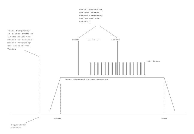
For both, the space or key-up tone for FSK CW may be placed anywhere convenient, but should avoid extending the span even further. Using the MGM sync tone for key-up when using the 800Hz option may offer a convenient value that keeps the aural listening environment uncluttered.
