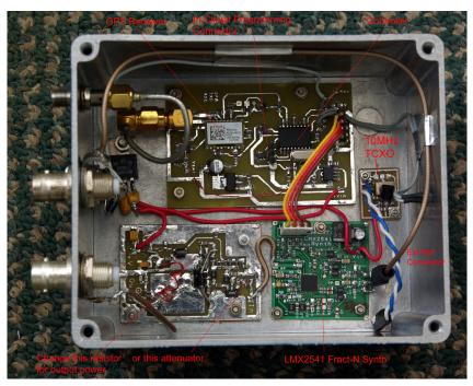
An LMX2541 based solution generating at 144MHz was used for both DLOSHF EME beacons where their outputs at 144MHz are mixed up to 10GHz and 24GHz. An early version of the hardware shown here.
