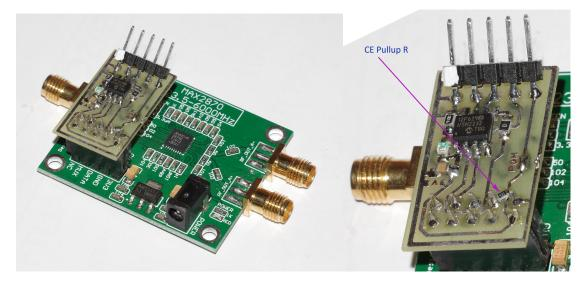
Photo 1 PIC + MAX2870 module PIC module in closeup, showing additional CE pullup resistor for MAX2870
