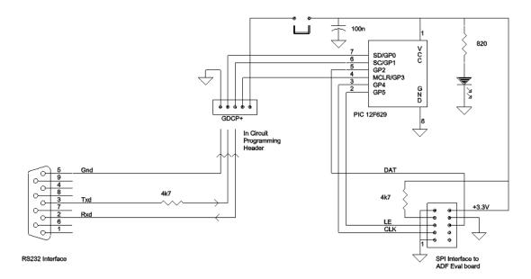
Figure 1 PIC module circuit diagram
