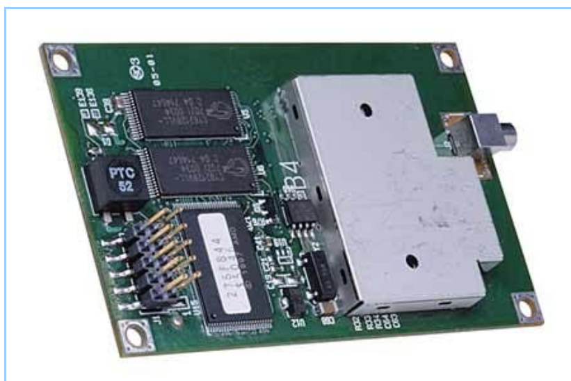
Figure 2 – The Jupiter-T GPS receiver
