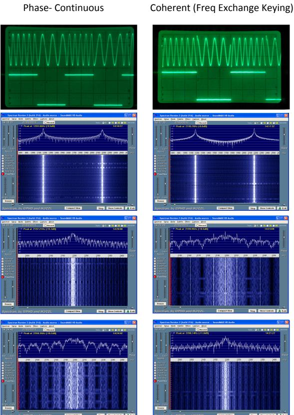
Both FSK signals shown on the spectral plots are 1200/2200 Hz tones switched with a 25WPM CW message for a random bit pattern. Frequency resolution, top to bottom for each pair of spectra are : 8Hz, 0.7Hz, and 0.18Hz. Latter two show the 2200Hz tone only. Waveforms are generated from PIC G4JNT PIC\_DDS source using code *freqsource* and cohfsksrc respectively.
