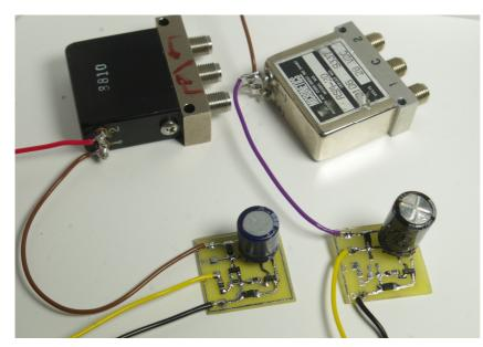
Two boards made up and connected to their respective relays. The one on the left is a Dynatech relay with a coil resistance of  $180\Omega$ . Although rated at 28V, it appears to pull-in at 14V and drops out at around 7V. In the doubling circuit here it works from a supply as low as 9V
