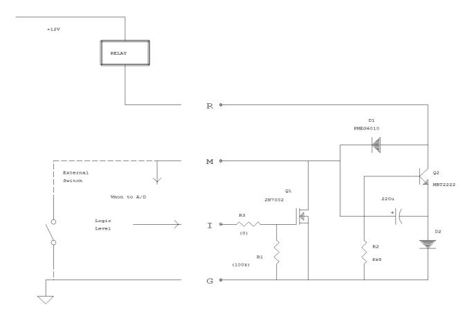
External connection nomenclature : [R]elay, [M]onitor [I]nput, [G]round. R1 is there to stop the input floating if left unconnected. R3 - just in case it may be needed. (It costs nothing to provide PCB pads and link them if unwanted but more effort to cut tracks and add them later). The value of R2 is not critical, D1 and D2 were just what I had available.
