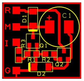
The design has the option for logic level drive (+5V Tx / 0V Rx) to the 'l' terminal or an external switch that may already be available can be connected to the 'M' terminal.
