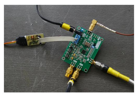
Default settings provided by Analog Devices design software . 10MHz reference input comes from a good quality TCXO and the reference doubler is enabled for a 20MHz Fcomp.
