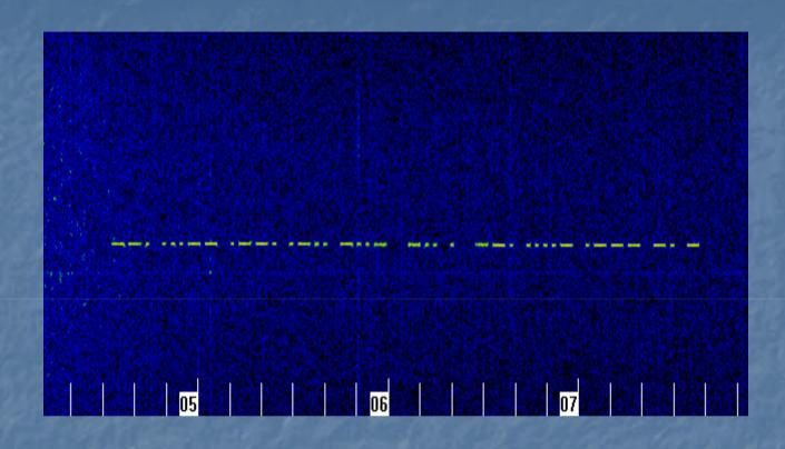
The first ever QRSS QSO on 73kHz 3 hours for two callsigns 0.04Hz bandwidth
