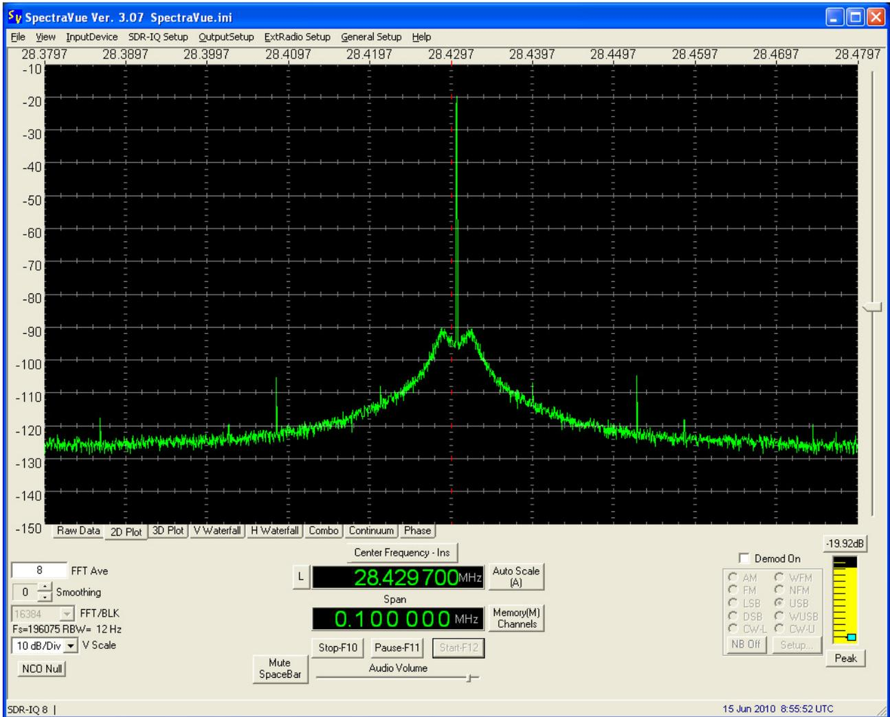
**Figure 5 Phase noise plot at Fcomp = 172kHz PLL BW = 6kHz**
