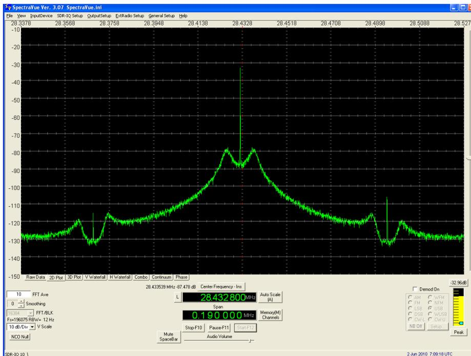
**Figure 2 Phase noise plot of initial PLL design**
