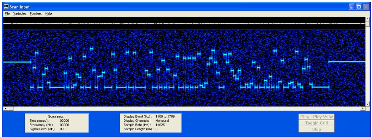
**Figure 6 Beacon transmitter spectrum while sending the JT65B sequence**
