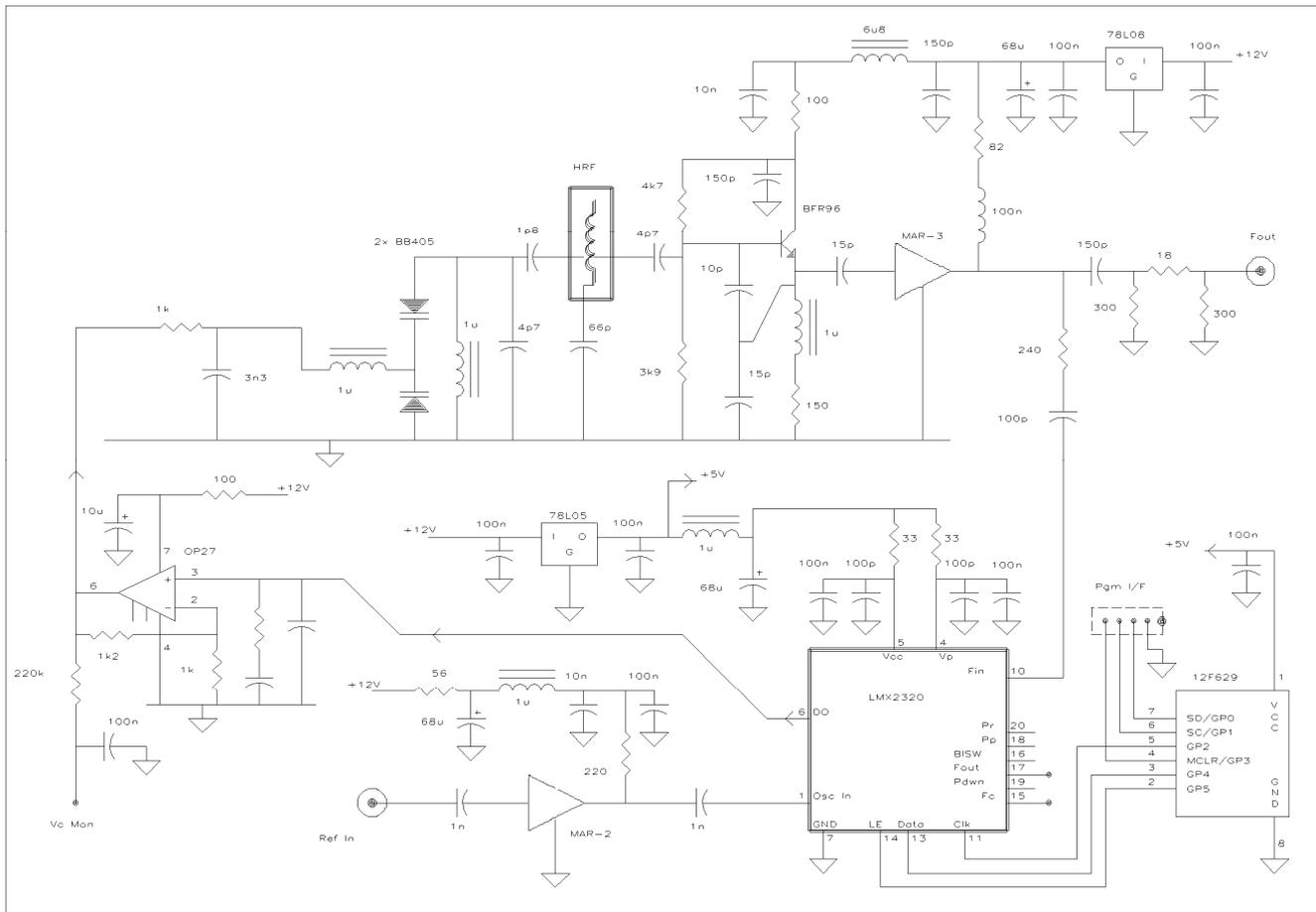
**Figure 3** Circuit diagram of final PLL
