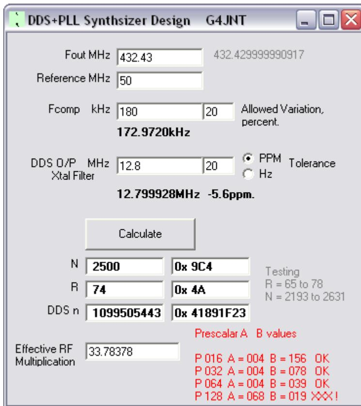
PLL filter values were calculated for a loop bandwidth of 16kHz which was about the widest that was possible with this VCO. To achieve a higher bandwidth required a higher tuning sensitivity on the VCO, and this was redesigned to the circuit shown in **Figure 3** where the bottom end varicap tuning was abandoned and a more conventional lightly coupled UHF varicap pair used instead. These have a higher Q and resulted in a marginal phase noise improvement in free run mode.
