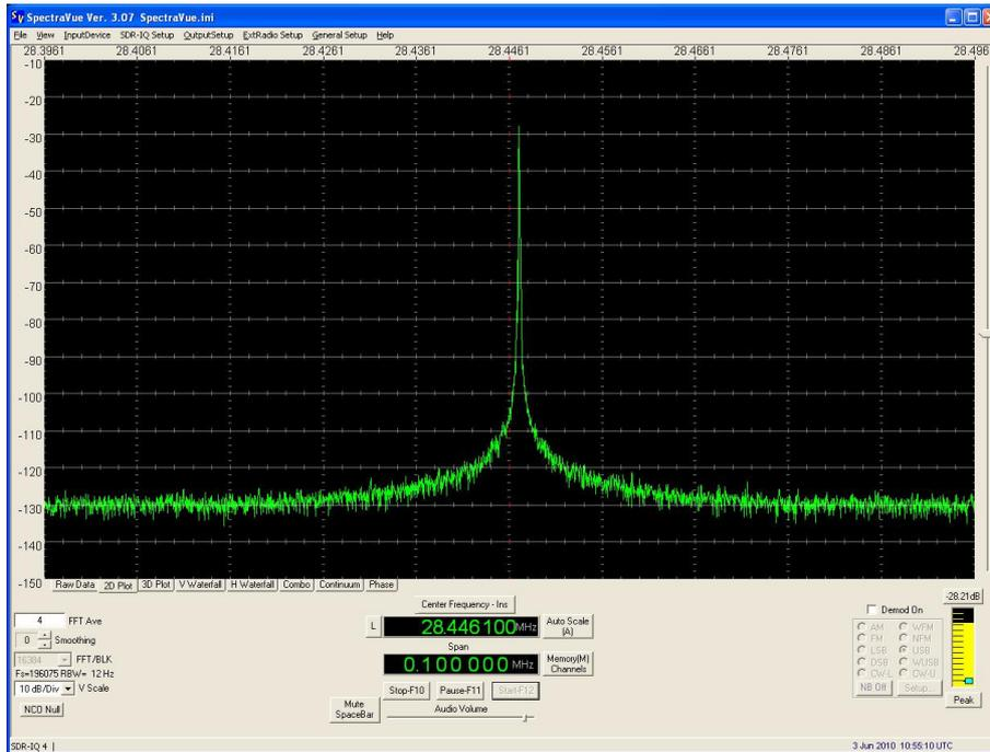
**Figure 1 Helical Resonator VCO - Free Running**
