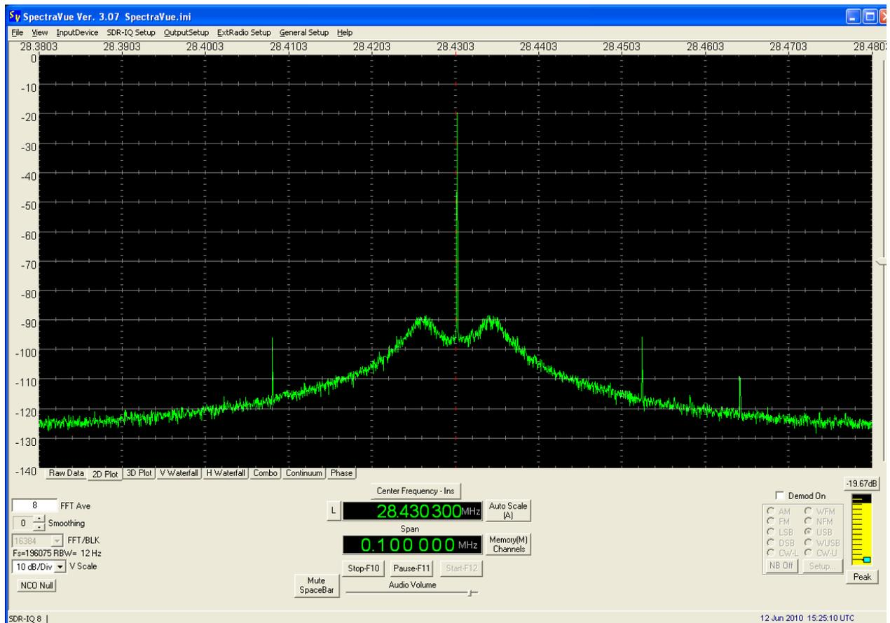
**Figure 4 Phase noise plot at  $F_{comp} = 172\text{kHz}$  PLL BW = 16kHz**
