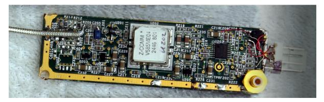
The output level from the synth at +15dBm was far too high for the AD8436, so 30dB of attenuation had to be added to bring it down to the drive level needed by that chip.
